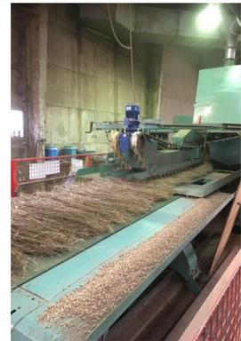
Figure 6: Breaking Machine
